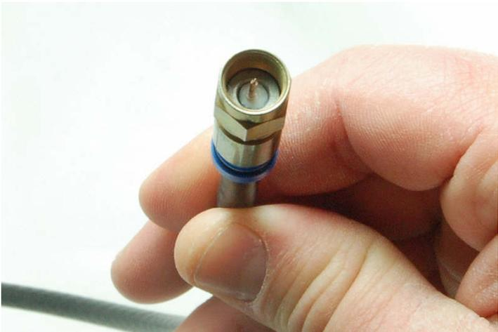
**STEP 8:** INSTALL THE CONNECTOR SO THAT THE CABLES WHITE DI-ELECTRIC COMES FLUSH WITH THE BOTTOM OF THE THREADS. THE INSTALLED FITTING SHOULD LOOK LIKE THE ONE SHOWN ABOVE.
