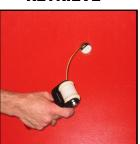
**INSERT** – Insert the leader magnet into the wall ( If insulated, ensure that the leader magnet is against the wallboard to secure a good connection with the retriever unit ).
