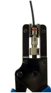
2. Insert your connector into your compression tool. The above pictured tool is the Holland Electronics CT-FBR.
