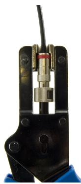
3. Squeeze the compression tools handle until the gap between the lower and upper connector halves is no longer visible. With Holland Electronics SLC connectors, there will be a pop and the end of the compression.
