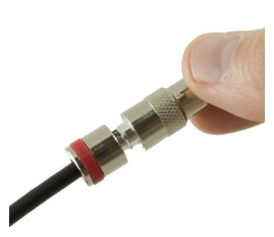
1. Once your Mini-Cable is properly stripped, you are ready to install your connector. It is very important to keep your connector perfectly straight with the cable. The cables center conductor has to meet a small opening inside the connector. If the connector is not installed straight your cables conductor will bend. The above pictured Holland connector has a window in the side to allow technicians to see when the connector is completely on (cable jacket appears in window).
