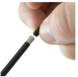
Next Remove the outer jacket from the second cut revealing the braid.
