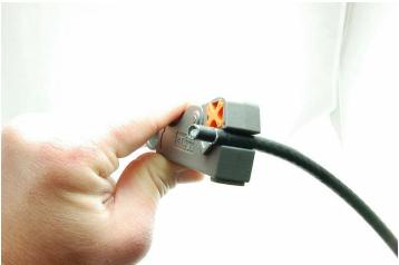
**STEP 4:** REMOVE THE CABLE FROM THE STRIPPER. BLADE DEPTHS CAN BE ADJUSTED WITH THE ALLEN SCREWS ON THE BOTTOM OF THE UNIT.
