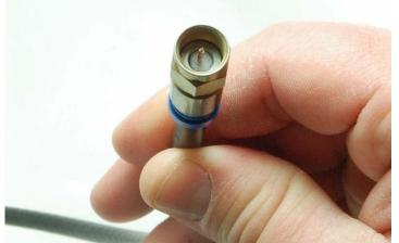
**STEP 8:** INSTALL THE CONNECTOR SO THAT THE CABLES WHITE DI-ELECTRIC COMES FLUSH WITH THE BOTTOM OF THE THREADS. THE INSTALLED FITTING SHOULD LOOK LIKE THE ONE SHOWN ABOVE.
