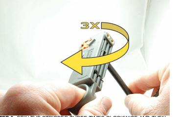
**STEP 3:** SPIN THE STRIPPER THREE TIMES CLOCKWISE AND THEN THREE TIMES COUNTER-CLOCKWISE.
