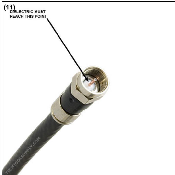
11. You are now ready to install your connector. Quad Shield RG6 cable requires special connectors that have a larger aperture on the back of the connector. Make sure the connectors you are installing are designed for Quad Shield RG6; if they are not, call Tech Tool Supply at 877-208-6657 and we will help you find the correct connector type for your cable.
