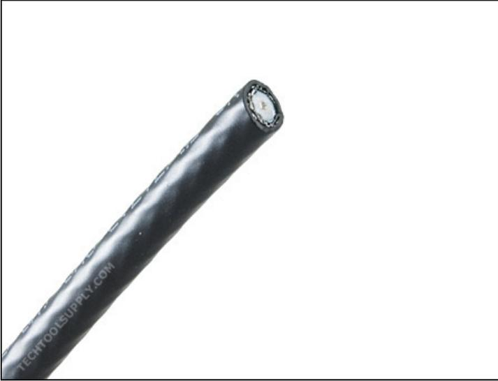
1. Quad Shield RG6 consists of the outer jacket (normally PVC or Teflon), an outer braid, an outer foil, an inner braid, an inner foil, the dielectric (white material), and finally the center conductor. In order to assure your cable stripper cleanly preps your cable, make sure that your cable was not smashed by your cutters. If your cable was misshaped or smashed when you cut it, reshape the cable with your thumb and fore finger.
