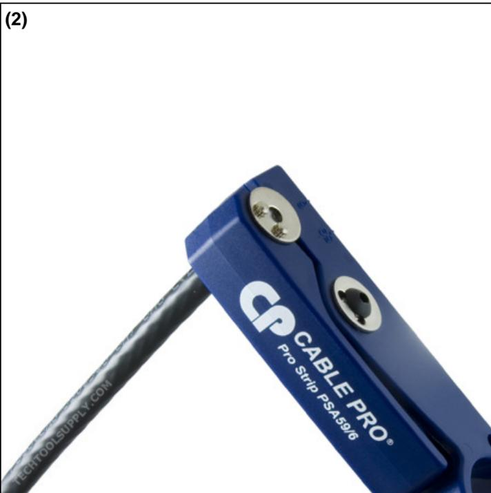
2. Insert your cable into your cable stripper. Every cable stripper is different; the Cable Pro PSA596 stripper pictured above has a built in cable stop so installers know when the cable is properly inserted..
