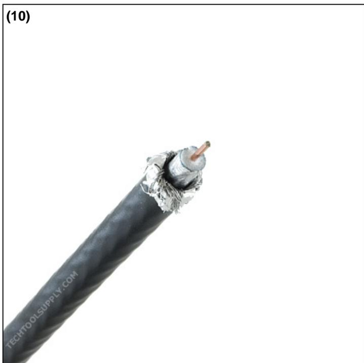
10. OPTIONAL: When properly done, your flared cable should look like the one pictured above. Notice how the flaring tool creates a perfect channel between the inner foil and the outer shielding. This allows for the connectors inner ferrule to slide down into the cable without any obstructions.
