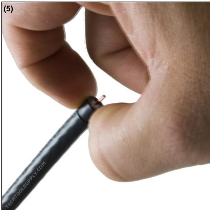
5. Using your thumb and fore finger, remove the first cable remnant which will reveal the cables center conductor. The second cut only scores the cables outer jacket.. Use your thumb and fore finger, or if necessary your wire cutters to pull this remnant off.
