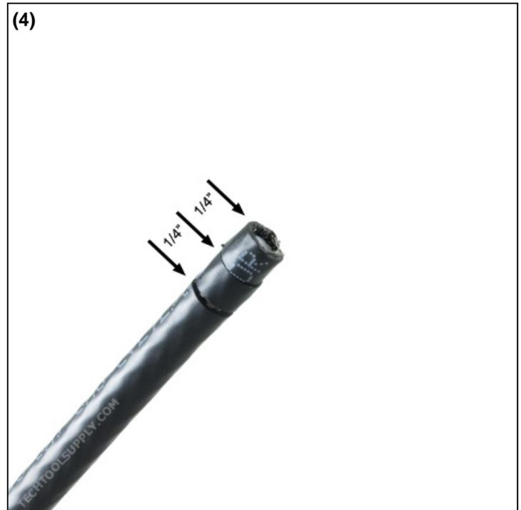
4. After you remove the cable stripper, you should have two different cuts 1/4" apart.
