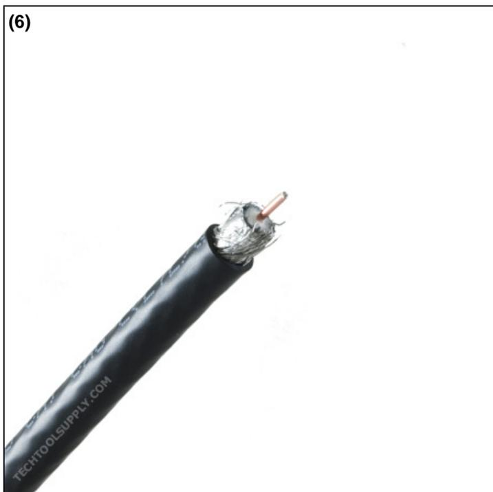
6. Your cable should resemble the cable pictured above. Notice how the outer braid in the picture above is undisturbed. If your cable stripper mangles or cuts the outer braid when stripping, you may need to adjust your stripper blades.
