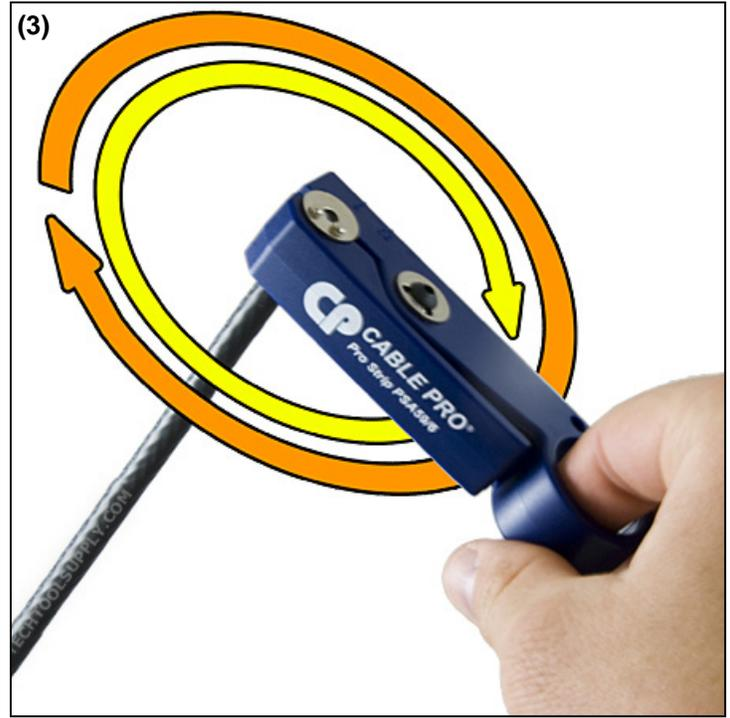
3. In a seamless motion, spin your cable stripper three times clockwise, and then back three times counter-clockwise. Squeeze the tail of your cable stripper and remove the stripper from the cable. We do not recommend using your cable stripper to remove the remnants. We've found that using your fingers to remove the cable remnants doubles the strippers blade life and provides a better connector installation.
