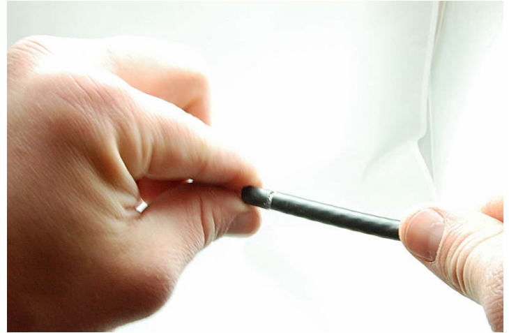
STEP 5: IT IS RECOMMENDED YOU PULL OFF THE COAXIAL CABLE REMNANTS WITH YOUR FINGERS TO EXTEND THE LIFE OF YOUR STRIPPER BLADES.
