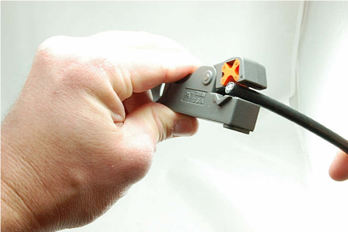
STEP 1: SET THE ORANGE V-BLOCK TO THE PROPER WIRE SIZE BY REMOVING IT, AND RE-INSTALLING IT WITH THE CORRECT SIZE.
