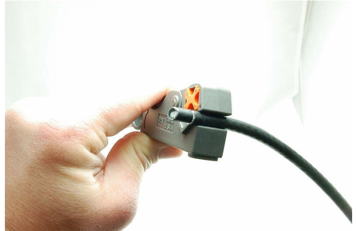
STEP 4: REMOVE THE CABLE FROM THE STRIPPER. BLADE DEPTHS CAN BE ADJUSTED WITH THE ALLEN SCREWS ON THE BOTTOM OF THE UNIT.
